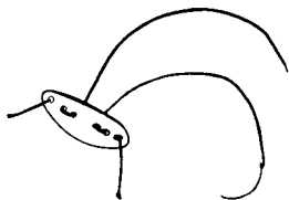
FIG. 1. Device for exteriorizing electrocardiograph leads. If required, cannulas may be exteriorized via the same device.
